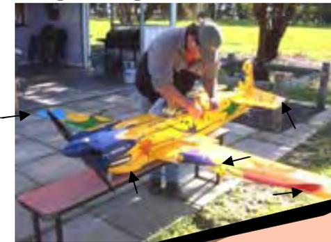
Clint had some engine problems and was coming in for landing but misjudged the tree on the western end of the runway. The CAP 580 'Splat' landed in the top of the tree (SPLAT!) and then fell through the tree which caused most of the damage to wings and elevators. The fuselage was undamaged except for a loose engine mount.
